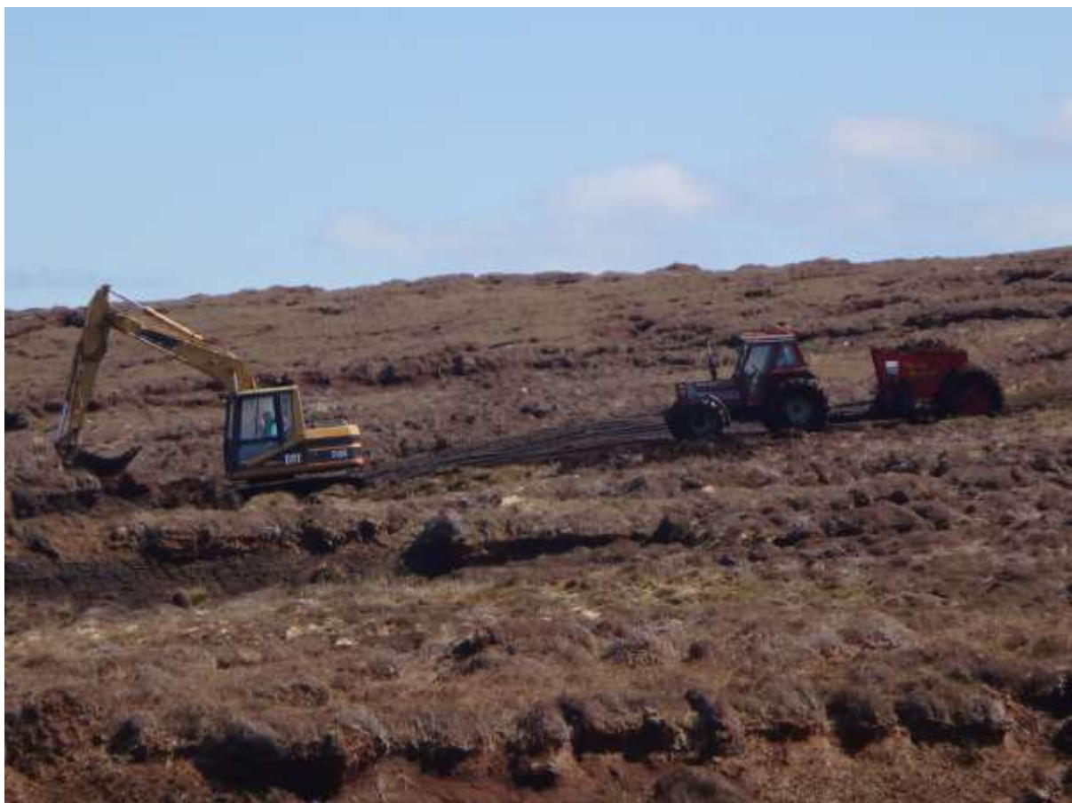
Figure 1: Extraction of turf using digger and hopper from Slieve Tooley SAC in Donegal in 2016. Photo: IPCC
