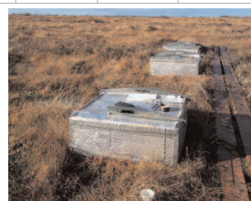
Figure 14: "Dark" chamber on Moyarwood Bog, Co. Galway used for measuring methane (CH 4 ) and nitrous oxide (N 2 O) fluxes. Photo: © D. Wilson
