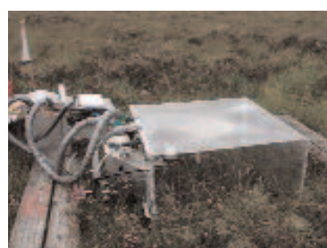
Figure 15: "Clear" chamber on Clara Bog, Co. Offaly used to measure net exchange of CO 2 between an ecosystem and the atmosphere (NEE). Photo: © D. Wilson
