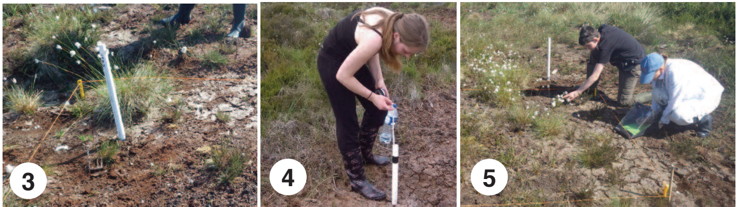
3: Home-made piezometers were installed to measure water levels in each plot and control area. Ideally the piezometer should be in a place for a year before restoration to give a complete picture of the water table levels from measurements taken each month. 4: A plover was used to determine water levels. This device makes a popping sound when it touches the water surface in the piezometer. 5: A 2mx2m quadrat was taken to record the vegetation present before restoration in all 4 plots and in each control area.
