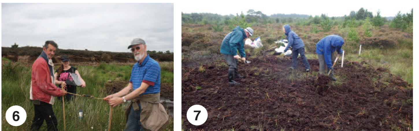
6: The plots were profiled to determine the slope. This information along with the water table depth determines how much peat must be removed from the bog surface. 7: The surface peat to a depth determined by water level and slope (varied from 5cm-20cm between plots) was removed by digging and raking and the material removed was piled up around the perimeter of the plot and control areas.
