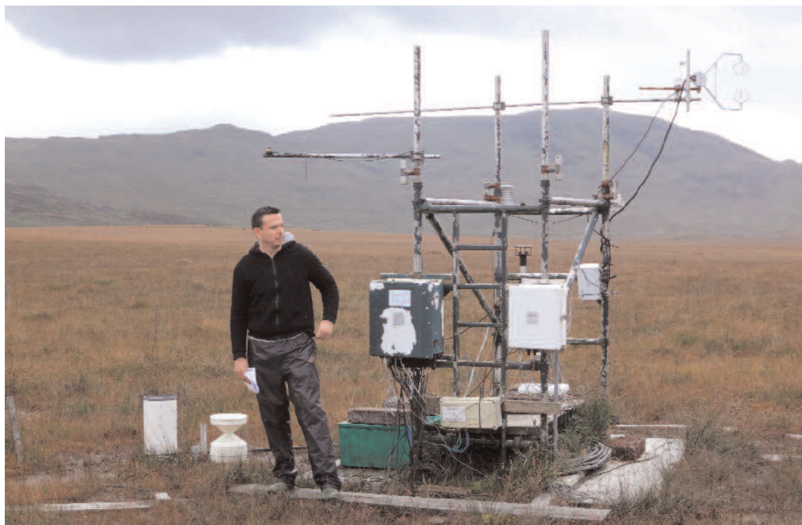
Figure 8: Greenhouse gas monitoring equipment on Glencar Bog SAC, Co. Kerry. This site was found to be sequestering carbon and had a total carbon sink balance of the order of -30 g C m -2 yr -1 . Photo: © C. O'Connell
